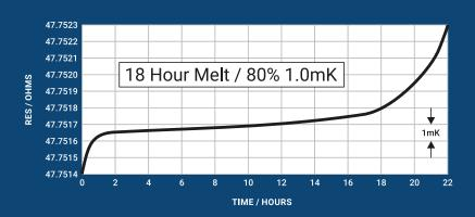
Plateau lengths at the silver point of over 70 hours (3 days) have been achieved using our furnaces. From a practical point we normally work with one working day long plateaus, re-melting the cell overnight ready for a new freeze the next day.
