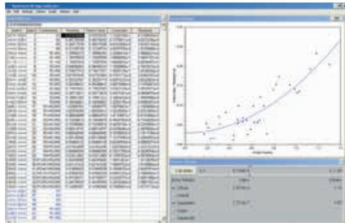
The combinatorial calibration method is particularly powerful because it is not necessary to know the actual values of the four resistors, or their frequency dependence. This means we can calibrate any ac or dc bridge to any accuracy, so long as the various resistance combinations are accurate.
