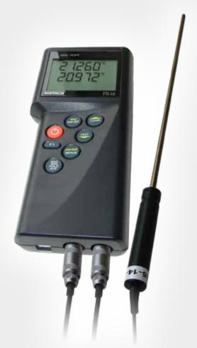
The TTI-10 brings laboratory level performance of up to 0.01°C (10mK) and resolution up to 0.001°C (1mK) in a portable handheld instrument. Battery life is typically 20 hours from a 9V PP3 alkaline battery and a protective rubber boot, that is included as standard, offers protection in field use.
