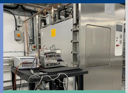
Decontamination of re-useable surgical instruments is classified as re-manufacturing under the Medical Devices Directive. The Directive is harmonised with equipment technical standards covering, EN 285:2015 details best practice for Steam sterilizers and for Washer Disinfectors EN / ISO 15883-1:2009 applies, Part 1 covers General requirements, terms and definitions and tests.
