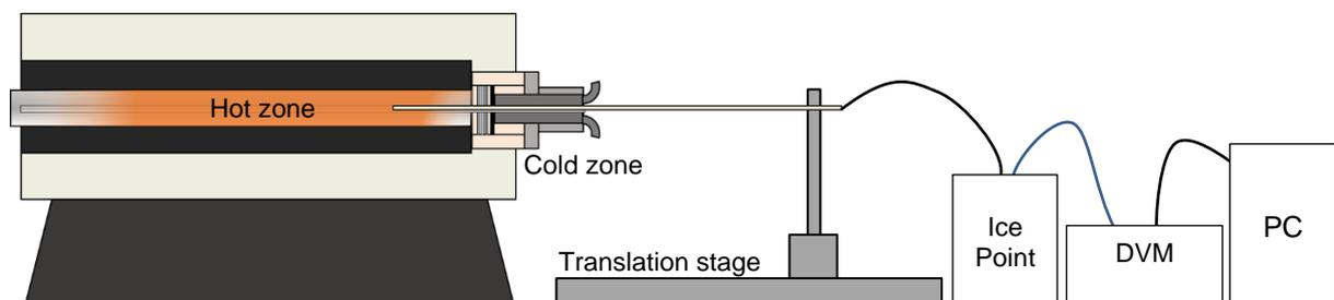
Figure 1 NPL’s homogeneity scanner and peripheral equipment.
