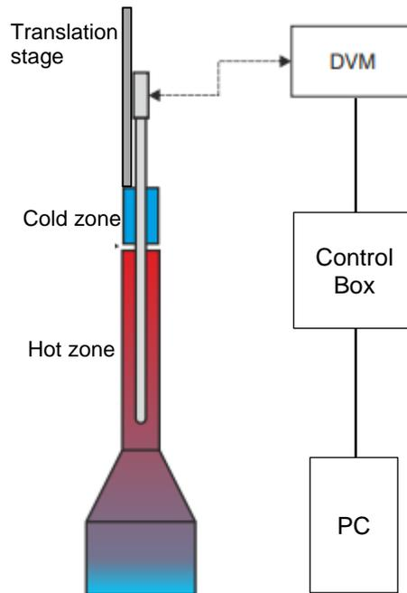
Figure 2 Isotech Homogeneity Scanner and peripheral equipment.
