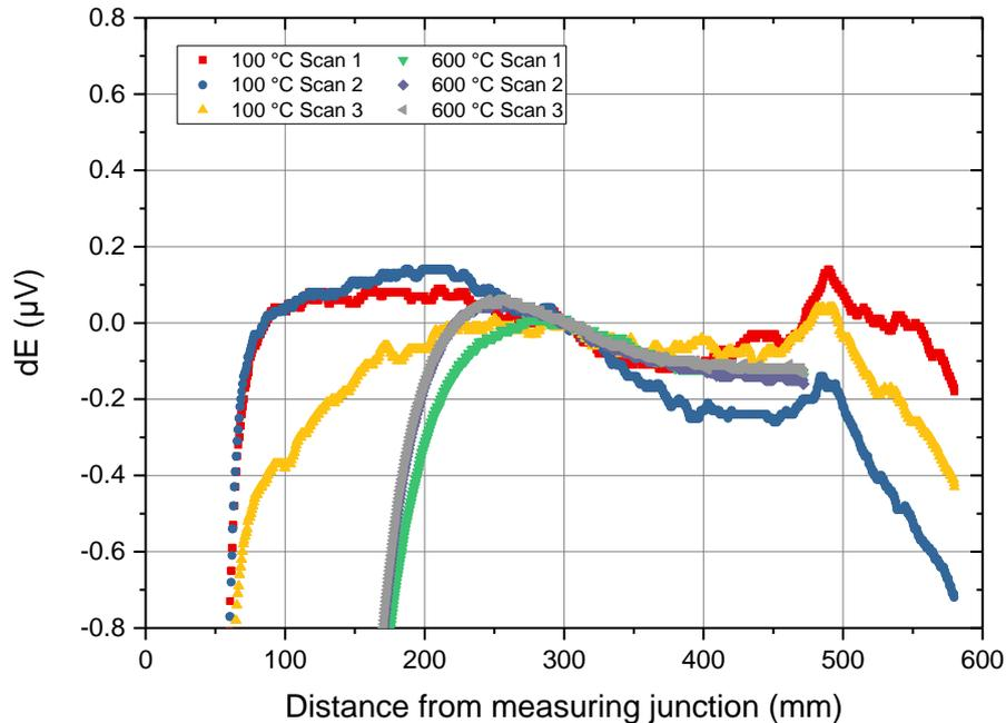
Figure 6 A graph of the homogeneity scans of the Pt-Pd thermocouple, where the x axis is the distance of the thermocouple tip from the sharp temperature gradient. The 100 °C scans were performed in the Model 881 and the 600 °C scans in the NPL scanner.
