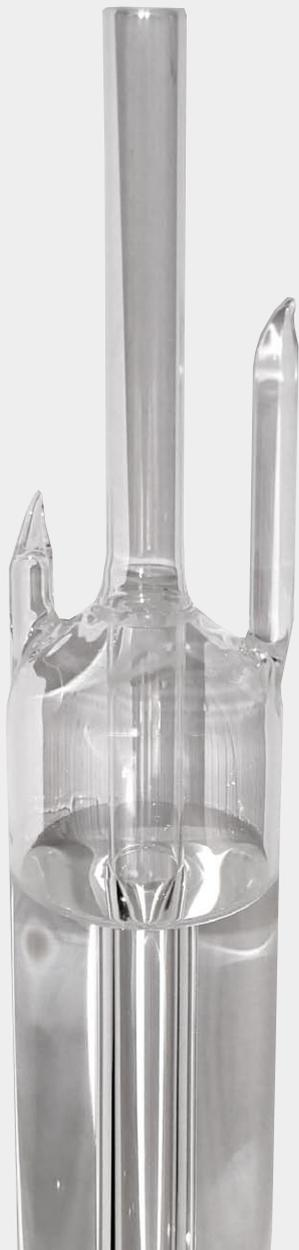
The Isotech-Jarrett cells have been in production since 1958. An independent comparison showed the first cell to be within 0.000006°C of the reference cell. The most recent international study organized by BIPM consistently shows labs using both recent and older Isotech-Jarrett cells tightly grouped, tens of µK around the BIPM reference value.
