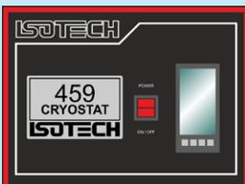
The Cryostat includes an external temperature control system that connects via 2M leads to the Cryostat Assembly.
