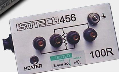
These devices have performance close to the superior SRA Models. A highest quality bulk metal film resistor is held in a temperature controlled environment that is heated to  $30^{\circ}\text{C} \pm 0.1^{\circ}\text{C}$ . Simply connect the Model 456 to a power supply and the resistor will warm up in typically 30 minutes and a LED shows when the temperature has been reached. A test pocket is provided so that the resistor's temperature can be monitored if required
