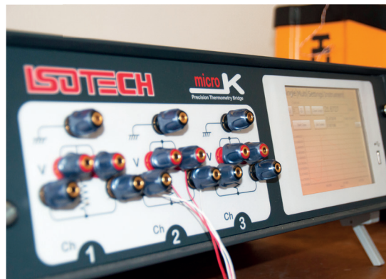
microK is drift-free in ratio measurement in contrast to older technology.
