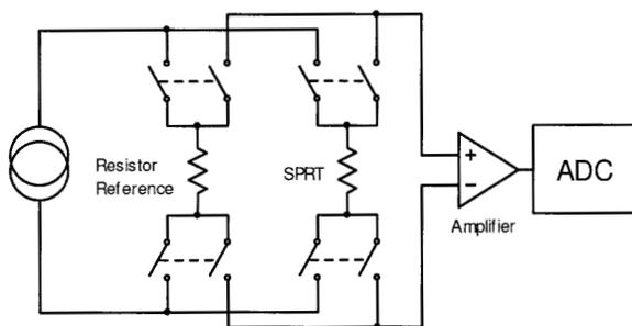
Figure 6. Substitution measurement topology.
