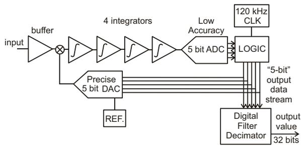
Figure 4.  $\Sigma$ - $\Delta$  ADC with 5-bit feedback.
