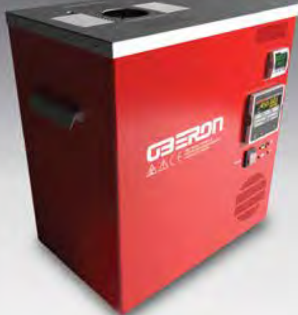
Oberon for Aluminium or Copper Slim Fixed Point Cells
