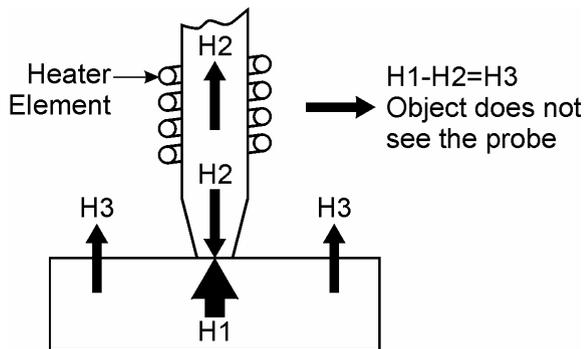
Figure 2. A Schematic of a Thermally Compensated Sensor.
