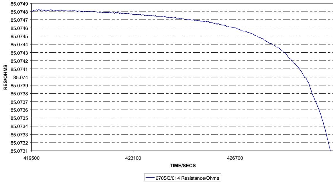
**Isothermal Tower Aluminium Fixed Point Cell MELT PLATEAU 5**
