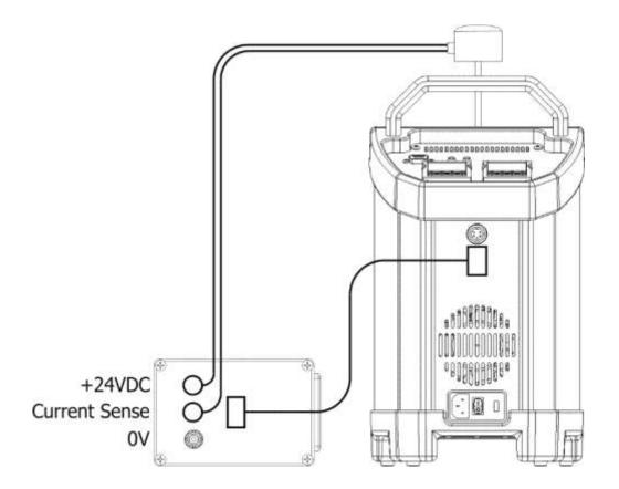
Connect the Transmitter to the equipment as shown in the above image.
